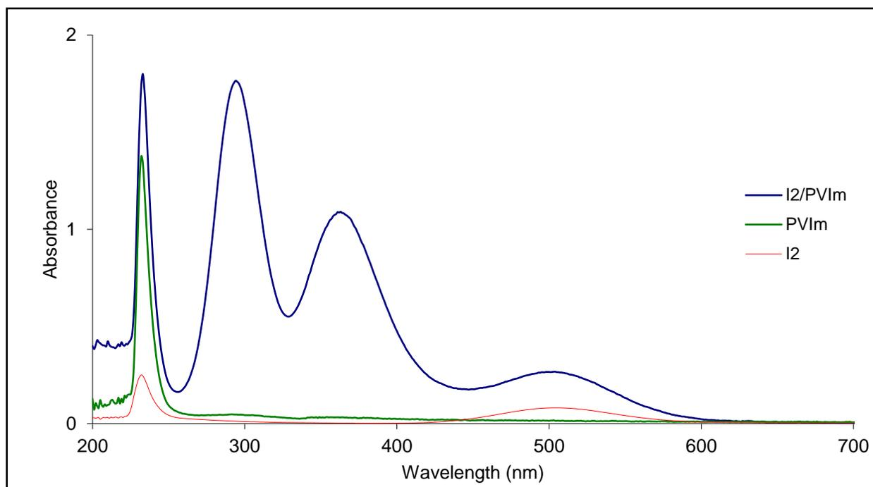
**Figure 2.** UV-visible absorption spectra of iodine, P(4VP), and  $[P(4-VPI)^+[I_3]^-]$  in dichloromethane.
